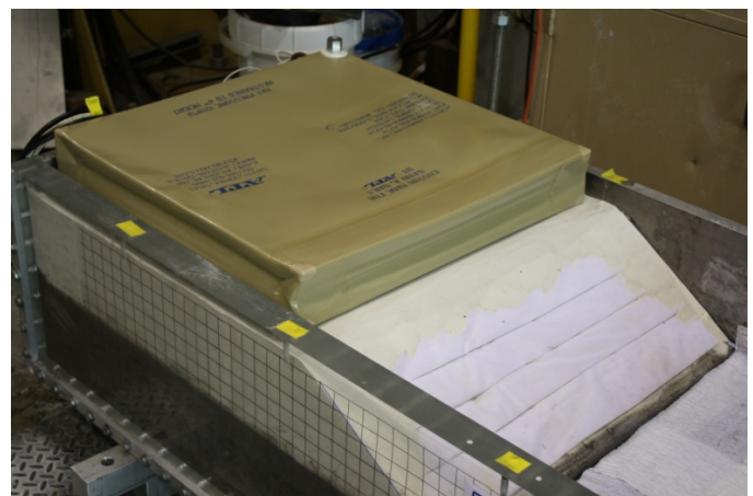
Figure 3. Custom-made air bladder on sand embankment.
