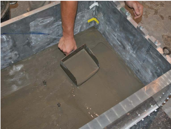
Figure 1. Placing fly ash slurry to form test bed deposit.
